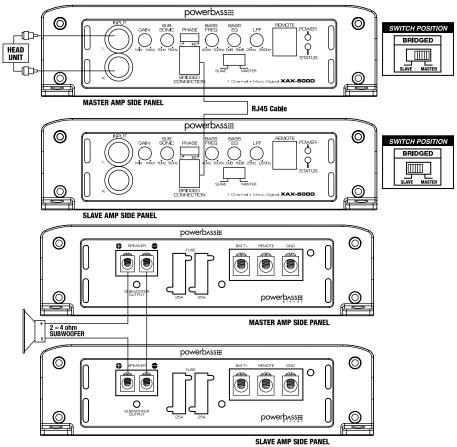
Fig.13 Dual Link minimum 2 ohm load
