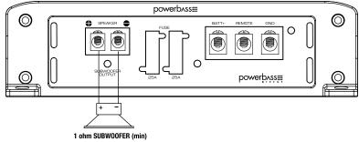
Fig.10 A Single Voice Coil Subwoofer (1~4 ohm)
