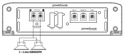
Fig.11 Two 4 ohm Subwoofers with Single Voice Coil
