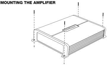
Fig.1 Mounting the Amplifier
