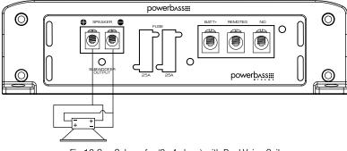
Fig.12 One Subwoofer (2~4 ohms) with Dual Voice Coil
