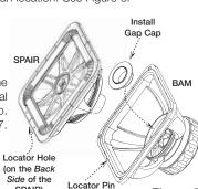
Install the Gap Cap around the BAM's pole-piece to protect the motor assembly from debris during the installation. Metal shavings would be nearly impossible to remove from the gap. Please protect your purchase, use the Gap Cap. See Figure 7.
