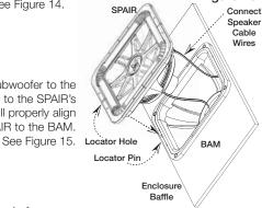
Pull the speaker cable wires (used to connect the subwoofer to the amplifier) through the BAM and connect them to the SPAIR's Binding Posts. The Locator Pin and Locator Hole will properly align the SPAIR to the BAM.
